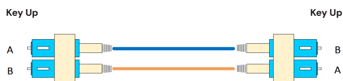
Diagram 1: A to B crossover patch cord
